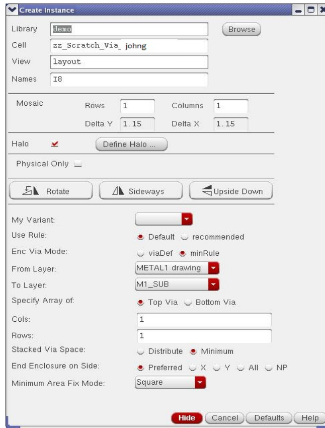
FIG. 18a create standard OA Via (using create instance interface)
