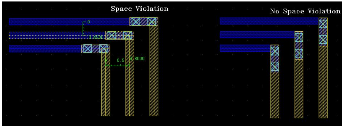
FIG 29d Corner via Spacing violations can be avoided by adjusting bus pitch and corner via alignment.
